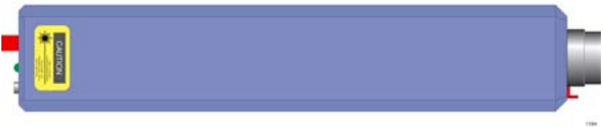
Figure 7. Top view of laser showing the location of the “warning logotype” label for a Class II laser.
